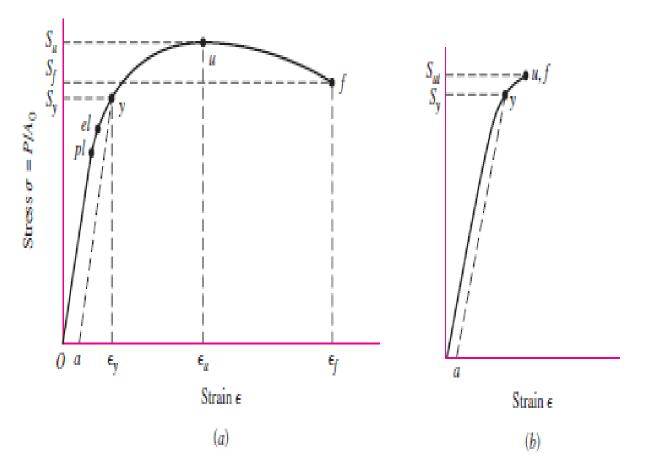
*pl* in Fig. 2–2*a* is called the *proportional limit*. This is the point at which the curve first begins to deviate from a straight line. No permanent set will be observable in the specimen if the load is removed at this point. In the linear range, the uniaxial stress-strain relation is given by *Hooke's law* as
