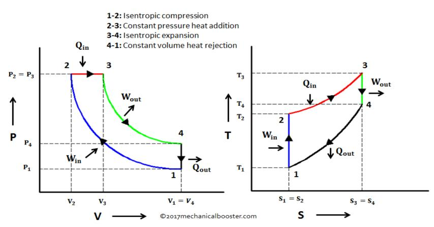
P-V and T-S Diagram of Diesel Cycle
