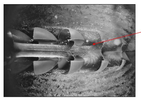
The buckets are shaped carefully to take advantage of the high momentum water jet, and are designed to turn around the water nearly 180° for maximum transfer of momentum from the water jet to the rotating turbine wheel.
