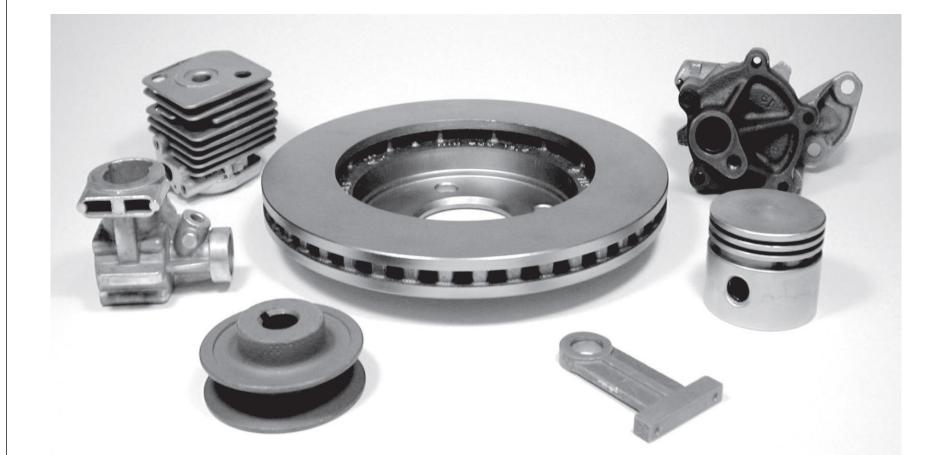
FIGURE 1 Examples of hardware produced by casting include a disk-brake rotor, automotive-oil, pump, piston, bearing mount, V-belt sheave, model-2airplane engine block, and a two stroke engine cylinder.
