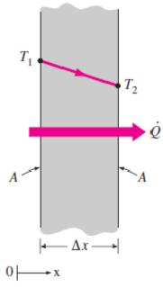
Thus we conclude that the rate of heat conduction through a plane layer is proportional to the temperature difference across the layer and the heat transfer area, but is inversely proportional to the thickness of the layer. That is,
