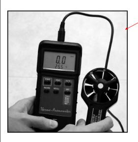
Turbine used for measurement of air speed
