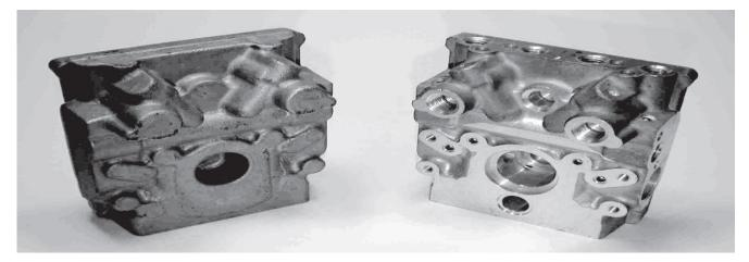
FIGURE 4: This body for a hydraulic valve assembly was first cast from aluminum (left) and then machined in order to produce holes, flatten surfaces, and cut threads (right).
