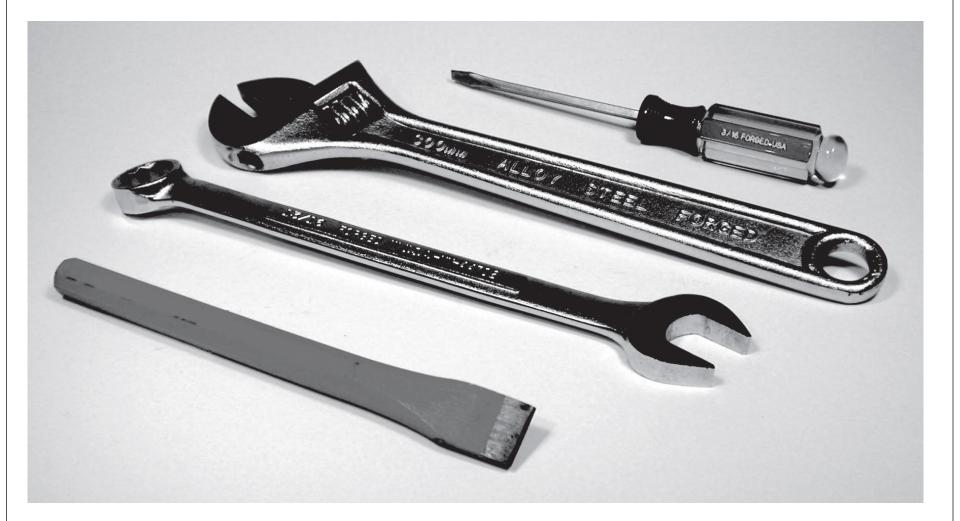
FIGURE 2: Examples of hardware produced by forging.
